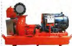
Dewatering Pump (Stationary)
