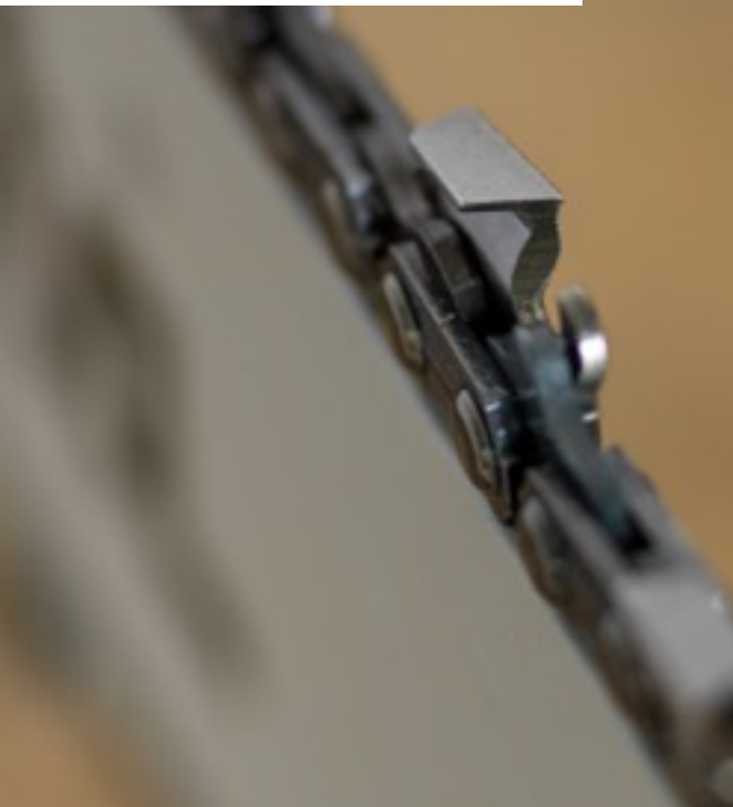
Correctly sharpened cutter
